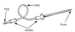
The temperature probe has a skewer-like probe at one end and a plug at the other end that goes into the outlet in the oven.
